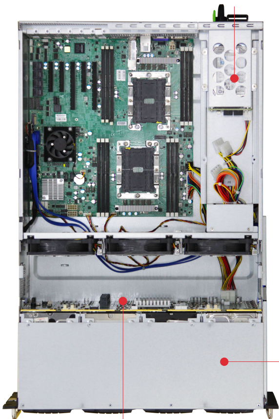
1 x 24-port 12Gb SAS backplane with 36-PHY expander chip and 3 SFF-8643 connectors
