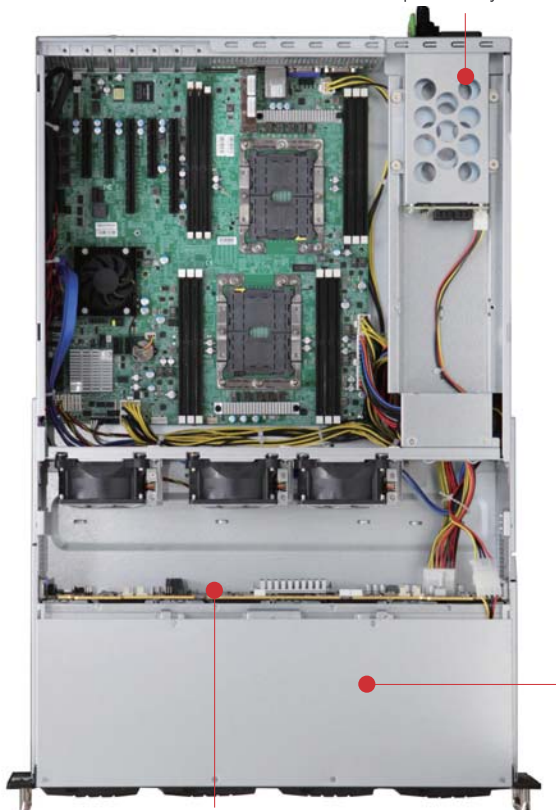
1 x 16-port 12Gb SAS backplane with 28-PHY expander chip and 3 SFF-8643 connectors
